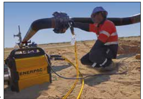
E-Pulse torque pump used for high volume fastening applications where weight is a critical factor. ▶
