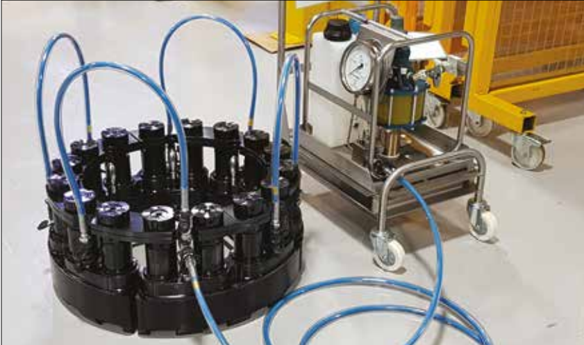
▲ Multi Stud Tensioning Set-Up.
