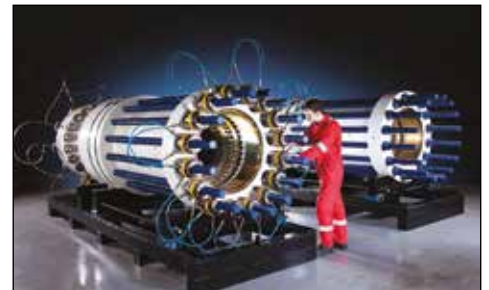
▲ Inter-connected with HT-Series hoses Enerpac subsea tensioners apply uniform bolt load.
