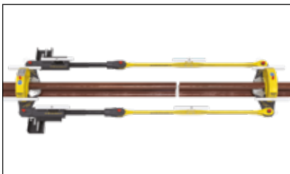
▲ Modular 70 ton stressor and holds the rail in neutral length during the welding process.
