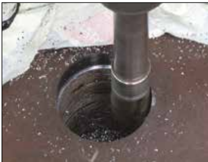
▲ Enlarging a hole
