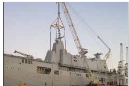
Synchronous hoisting and load positioning
