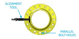
2. Insert the bolt into the aligned bolt-hole and release the alignment tool. The load will transfer onto the bolt.
