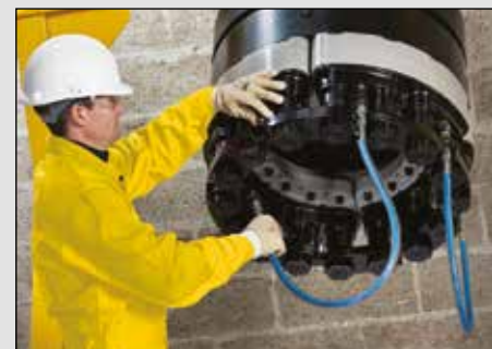
▲ Multi Stud Tensioning application.
